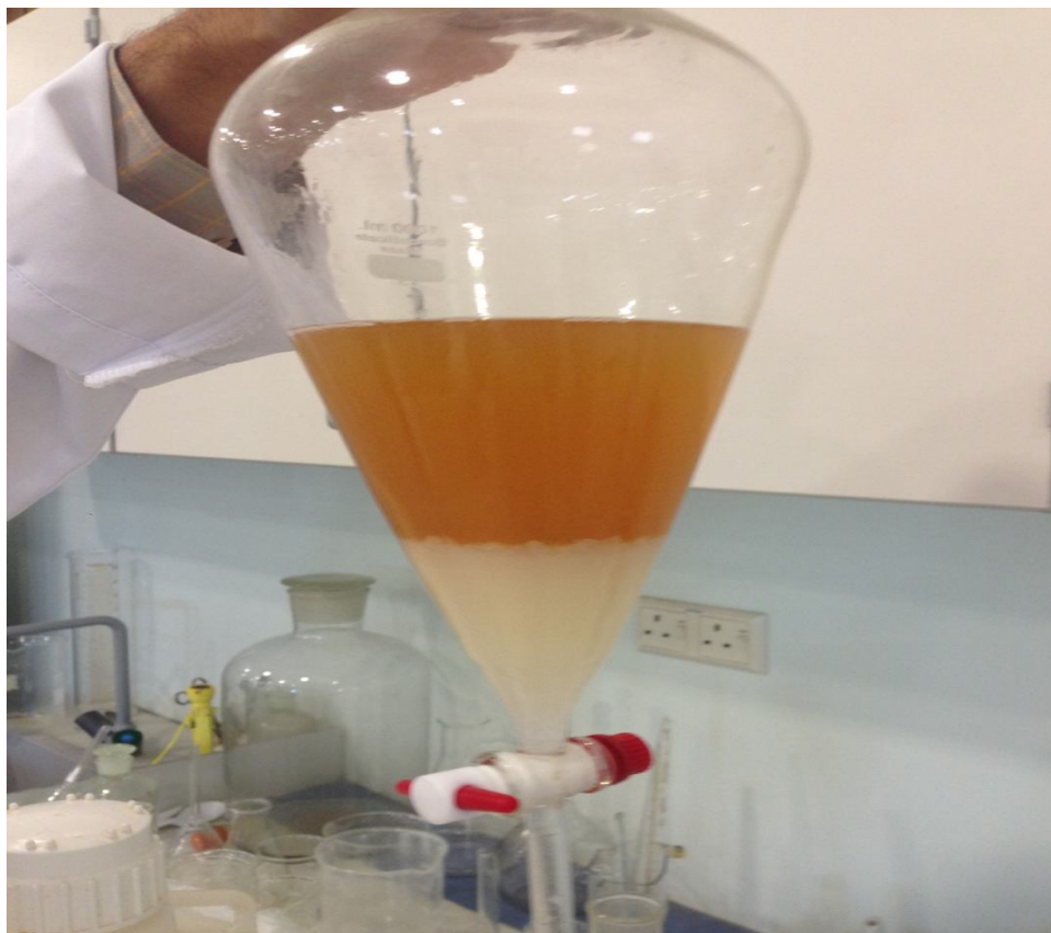
Fig. 2. Separation of antimicrobial compounds with using separation funnel.
